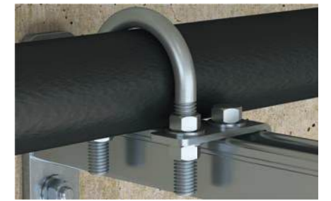
Pipe on cantilever arm with U-bolt ETR and channel connector FETR-C
