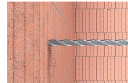
Drilling in perforated brick
