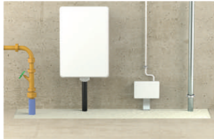
Mixed penetration through the floor
