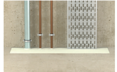
Mixed penetration through the floor
