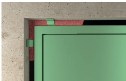
Back filling material
