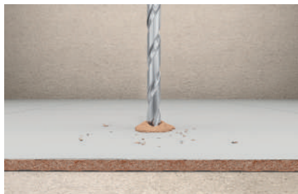
Drilling the material combination tile and concrete
