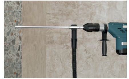
Cross section hollow drill bit
