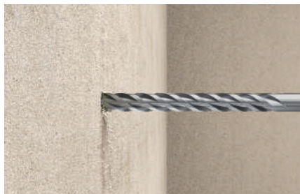
Drilling in masonry
