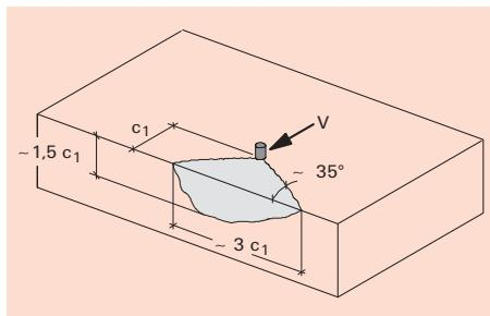
Figure 2.15 shows the concrete failure load  $V_u$  of fischer Zykron anchors subject to shear load in non-cracked concrete in relation to the edge distance  $c_1$ . The increase in the concrete failure load is a function of the edge distance to the power of 1.5, and is restricted again by the anchor's steel failure load.
