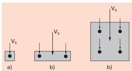
For the design proof of concrete edge failure (generally decisive for anchor groups with small concrete edge distance which are loaded towards the edge) it shall be assumed that only the most unfavourable anchor/s take up the shear loads. Examples are shown in Figure 4.2.
