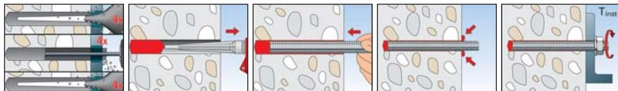
$d_0 \geq 18$  mm with oil free compressed air ( $P > 6$  bar)
