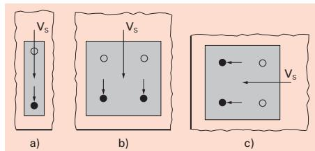
If the concrete edge distance is large ( $c \geq \max(60 d_{\text{nom}}, 10 h_{\text{ef}})$ ) it can be assumed that concrete edge failure is not decisive. In this case the design proof for concrete edge failure can be omitted.
