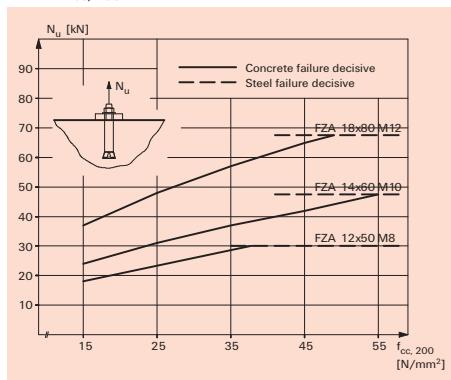
Figure 2.10 shows the relationship of the concrete failure load of fischer Zykron anchors in non-cracked concrete under shear load and the concrete cube strength  $f_{cc, 200}$ . This illustration is valid for anchors that have an edge distance  $c_1 = 80$  mm which are loaded towards a free edge.
