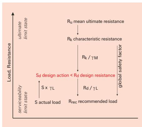
The partial safety factors for actions  $\gamma_L$  cover uncertainties and scatter of the dead and variable loads. The partial safety factors for the material resistance include scatter of the material resistance, namely the load bearing capacity of the fastening. The partial safety factors for the resistance depend on the quality and the failure mode (i.e. steel failure, pull-out failure, concrete cone failure) of the anchors.
