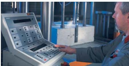
Tension test machines with various load attachments allow tension tests in small specimens (figure 2.24) or in large concrete elements (figure 2.25) also in cracked and non-cracked concrete. The load can be continually applied (force-controlled or displacement-controlled) and as either static, dynamic shock or fatigue load.
