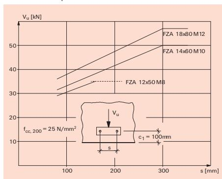
The failure load of an anchor pair increases with increasing anchor spacing until the spacing reaches 3 times the edge distance. For larger anchor spacing, no further increase in ultimate load can be expected because the maximum capacity of the anchor pair cannot exceed twice the maximum failure load of a single anchor with the same edge distance. For the fischer Zykron anchor FZA 12x50 M8, the maximum load bearing capacity of the anchor pair is limited by the steel failure load.
