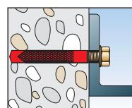
$d_0 \geq 18$  mm with oil free compressed air ( $P > 6$  bar)
