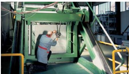
A parallel crack testing machine conducts tests in static and dynamic cracks.
