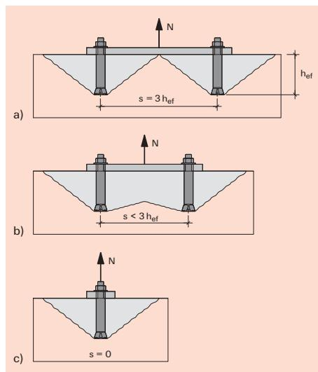
Figure 2.17 shows the effect of the anchor spacing for a pair of fischer Zykron anchors subject to axial tension load in non-cracked concrete with a strength of  $f_{cc, 200} = 25 \text{ N/mm}^2$ . The horizontal axis shows the ratios of the axial spacing to the anchorage depth.
