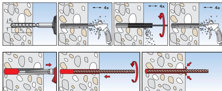
$d_0 \geq 18 \text{ mm}$  with oil free compressed air ( $P > 6 \text{ bar}$ )
