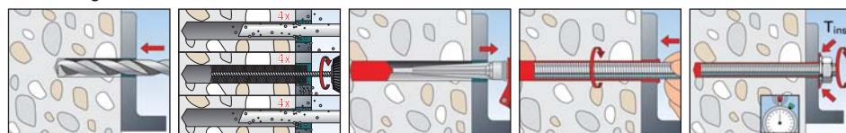
$d_0 \geq 18 \text{ mm with oil free compressed air } (P > 6 \text{ bar})$
