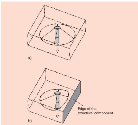
The figure shows an increase of ultimate load with increasing edge distance. When the edge distance exceeds  $c_1 = 75, 90 for FZA 12x50 M8, FZA 14x60 M10 and FZA 18x80 M12 respectively which corresponds to 1.5 times the anchorage depths or the radius of the break-out cone, no further increase in the failure load can be expected. This is because the break-out cone can deve-$
