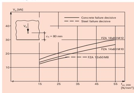
As with tension load, the ultimate shear load at concrete edge and pry-out failure is also dependent on the square root of the concrete strength, and is limited by the anchor's steel strength.
